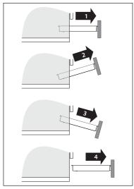
Figure 5b Removing the drawer
